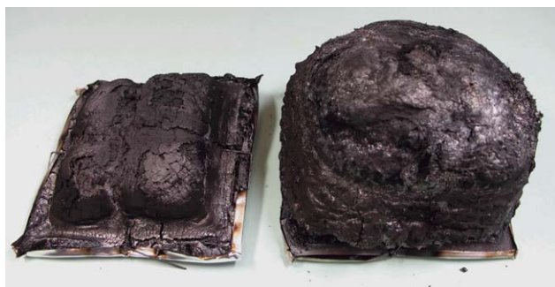
Figure 4. Fire residues after cone calorimeter measurements of EP + MPZnP (left) and EP + MPP (right). [Color figure can be viewed in the online issue, which is available at wileyonlinelibrary.com .]
